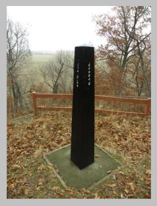
On December 6, 2014, a static GPS observation on the Cast Iron Monument located on the state line between Rulo, Nebraska and White Cloud, Kansas, was performed. A Topcon Hiper V receiver was used for the 4 hour-34 minute continuous observation. A 10'-5" tall tripod was used to center over a punch mark on the top of the Cast Iron Monument. The receiver was centered over the point by use of an optical tribrach and checked with a plumb bob. The file was then submitted to OPUS for processing.
